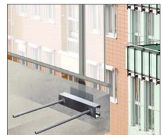
Attachment of railings
